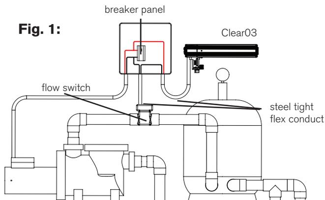
**The ClearO3 unit is factory set to 240VAC. The ClearO3 should be wired to run with the filter pump which creates the air draw through the unit needed to create ozone. Do not set the ClearO3 to run when the filter pump is off.**
